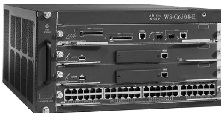
Figura 22. Switch Cisco Catalyst 6504-E
